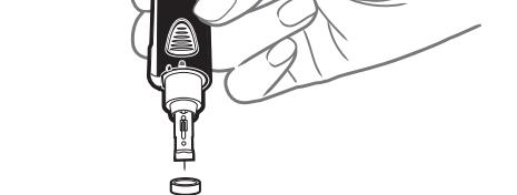
5. Attach and lock the endcap. Twist the white band to lock.
